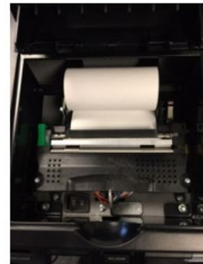
5. Press green lever toward you (level position)
